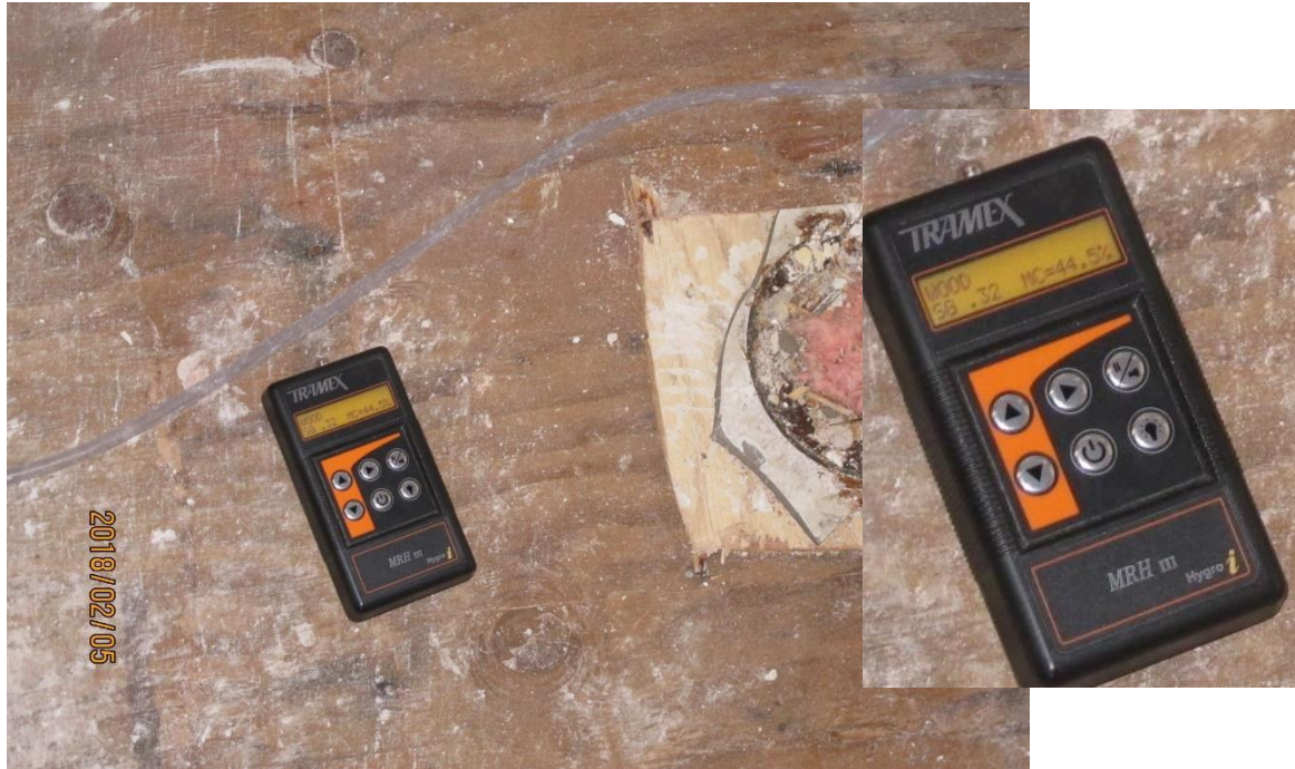
Unacceptable reading of 44% MC in utility room subfloor
