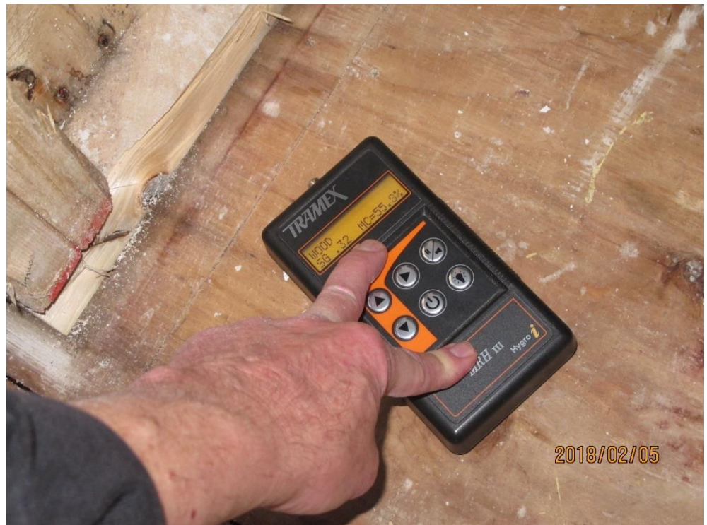
Unacceptable reading of 44% MC in utility room subfloor
