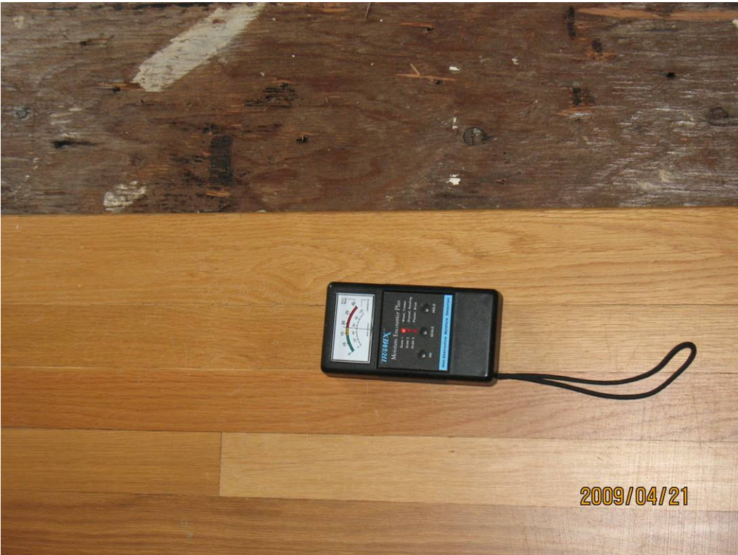
MM reading still marginal at 15+% MW near edge of kitchen step into dining room
